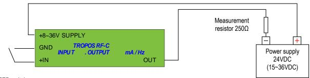
REED switch Example: Anemometer
